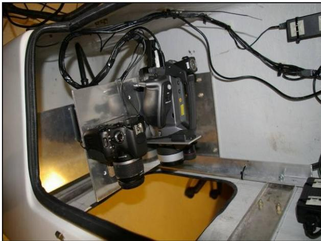
**Figure 3 : Helipod showing cameras in image capture position**
