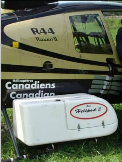
Figure 6 : Helipod attached to R44
