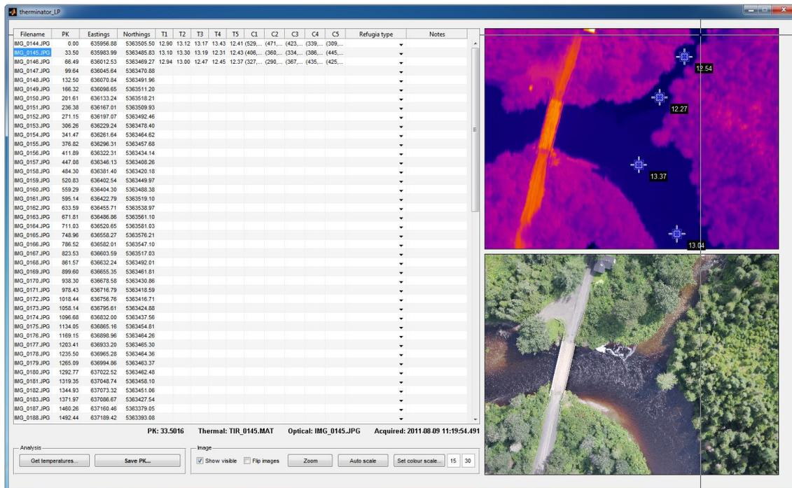
Figure 9: GUI (graphical user interface) used for the extraction of temperature measurements and the classification of thermal refuges from optical and thermal infrared images.
