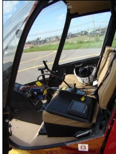
Figure 5 : Pan-tilt control panel
