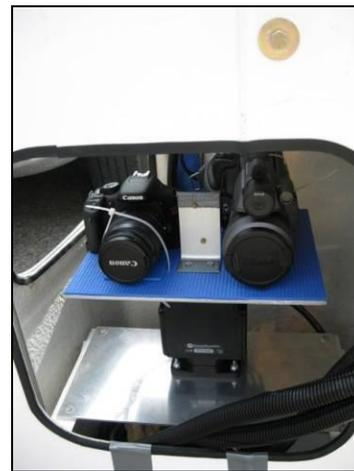
**Figure 4 : Optical camera (Canon) on left; TIR camera (FLIR) on right**
