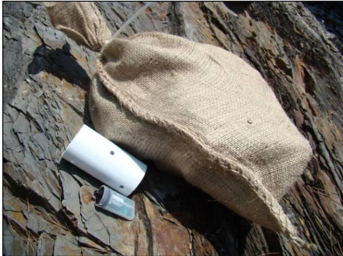
Figure 2 : Thermograph fixed in a UPVC tube (to protect from overheating and collisions with bedload), then anchored to a jute sack filled with rocks.
